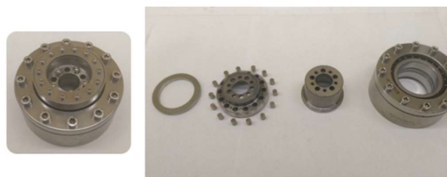
Figure 1 – Views of the unloading mechanism using SMA actuators
