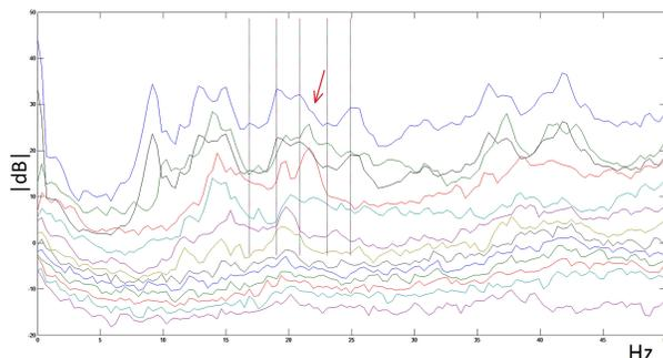
Figure 11. Tracking of mode at 22.71 Hz.
