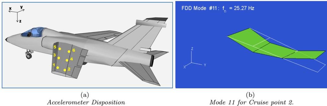
Figure 10. FDDT on a third generation aircraft
