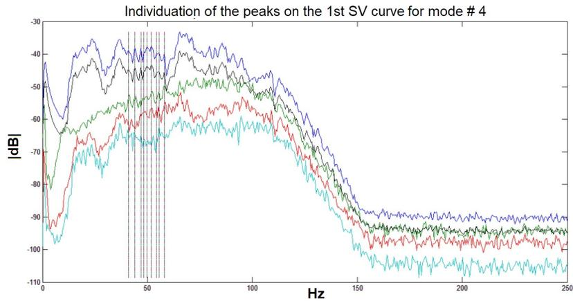
Figure 8. Example of selected frequency lines for the tracking of Mode 4.
