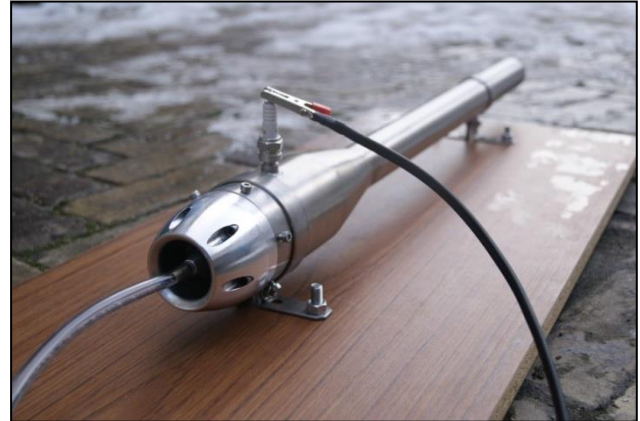
Figure 2. Pulsejet engine built by members of Association. 1
